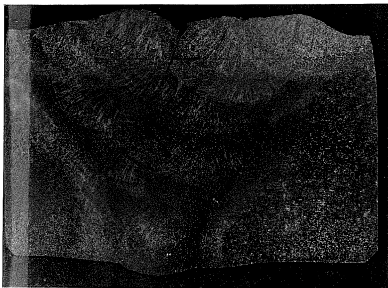
Figure 4-8 Cross Section of Fatigue Crack Initiating Between Weld Passes
